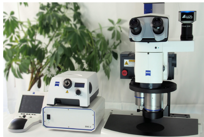
Zeiss V20 microscope with DeltaPix Camera and software
