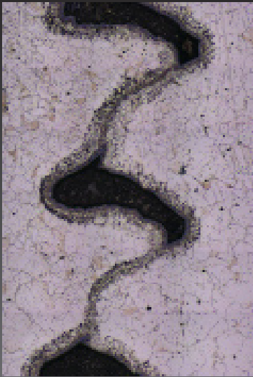
6x4 Auto stitched image captured with a 10x XYZ mono-zoom system and an Infinity X-32, showing a cut of a screw hole with a screw exposed to high temperature. Full overview is provided and details less down to 0.5 micron is resolved. Captured by "Haldor Topsoe".
